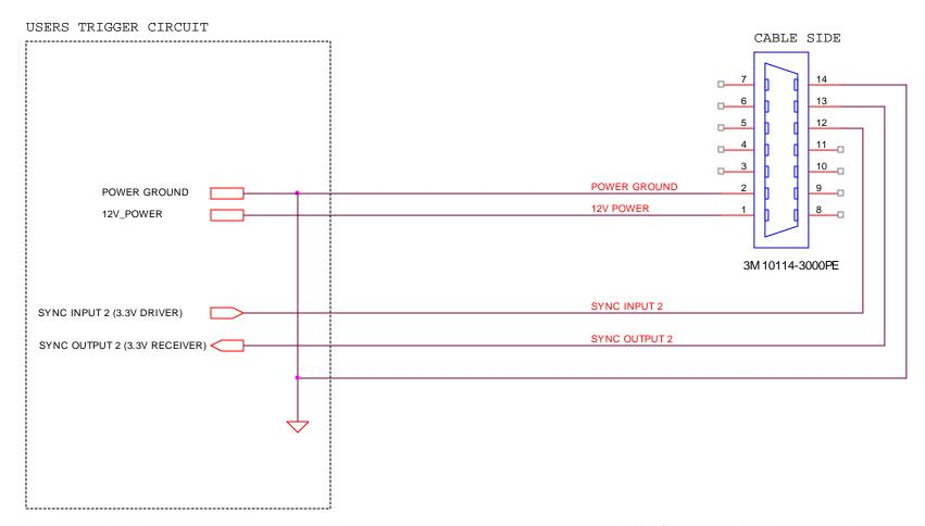
The non-isolated trigger circuit is connected to a Texas Instruments SN74LVC2G241 buffer/driver inside the camera. The required sync input current is less than 10uA and the maximum sync output current is 24mA. See the Texas Instruments SN74LVC2G241 for more detailed information.
