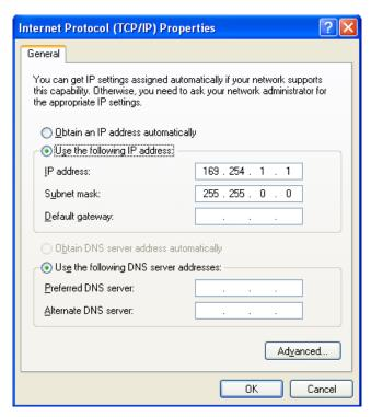
Figure 5. Network card TCP/IP address.
