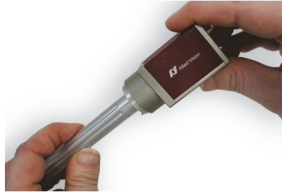
Figure 3: Removing IR cut filter/protection glass using special tools (P/N: E9020001 for 16mm filter and P/N: 3851 for 22 mm filter)
