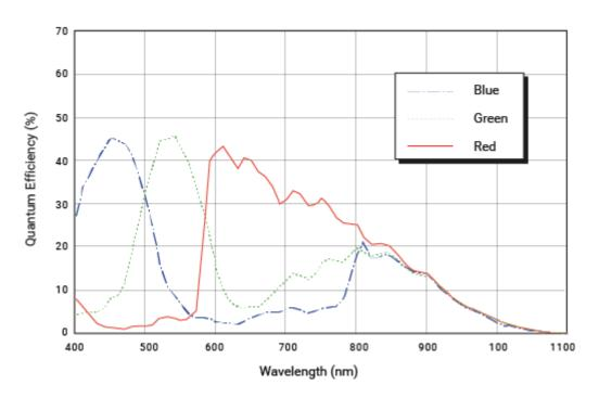
The spectral response curve excludes lens characteristics, light source characteristics, and IR cut filter characteristics.
