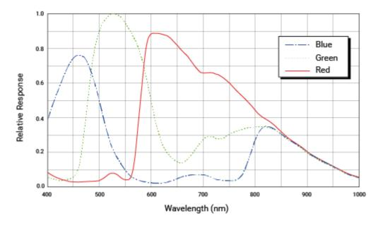
The spectral response curve excludes lens characteristics, light source characteristics, and IR cut filter characteristics.
