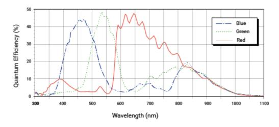
The spectral response curve excludes lens characteristics, light source characteristics, and IR cut filter characteristics.
