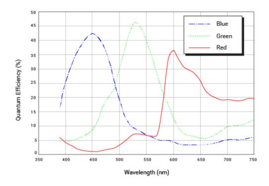
The spectral response curves exclude lens characteristics, light source characteristics, and IR cut filter characteristics.
