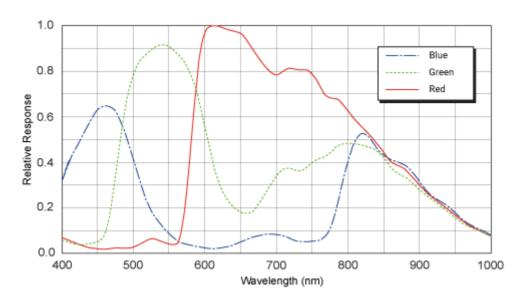
The spectral response curve excludes lens characteristics, light source characteristics, and IR cut filter characteristics.
