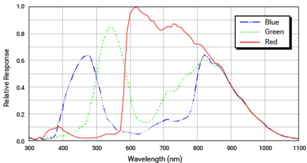
The spectral response curve excludes lens characteristics, light source characteristics, and IR cut filter characteristics.
