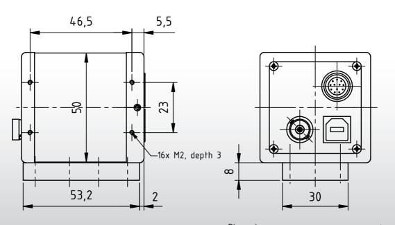
Dimensions: mm Tolerances: DIN ISO 2768m
