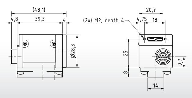
Dimensions: mm Tolerances: DIN ISO 2768m
