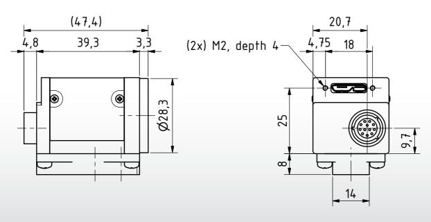
Dimensions: mm Tolerances: DIN ISO 2768m
