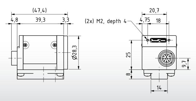
Dimensions: mm Tolerances: DIN ISO 2768m
