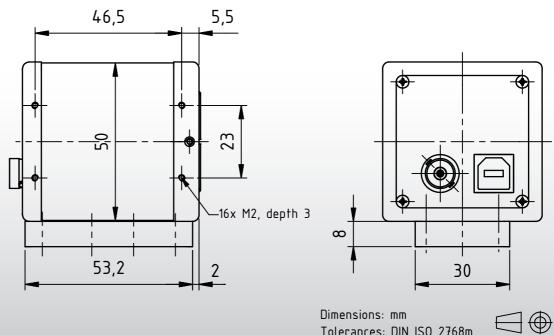
Dimensions: mm Tolerances: DIN ISO 2768m
