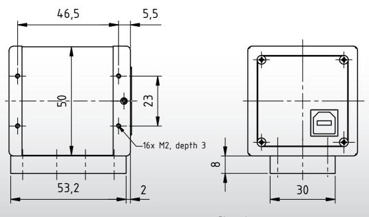
Dimensions: mm Tolerances: DIN ISO 2768m
