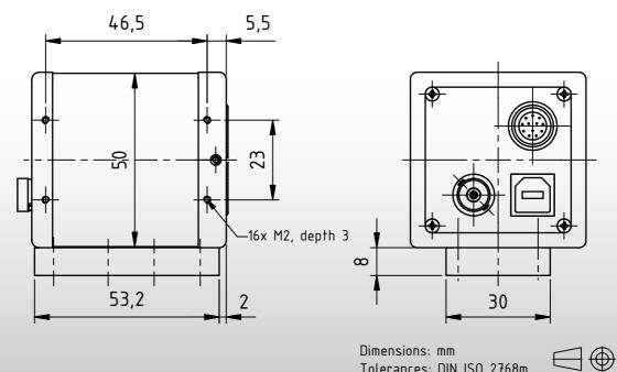
Dimensions: mm Tolerances: DIN ISO 2768m
