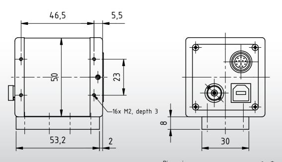
Dimensions: mm Tolerances: DIN ISO 2768m
