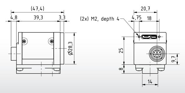
Dimensions: mm Tolerances: DIN ISO 2768m
