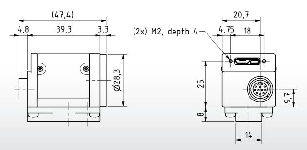
Dimensions: mm Tolerances: DIN ISO 2768m
