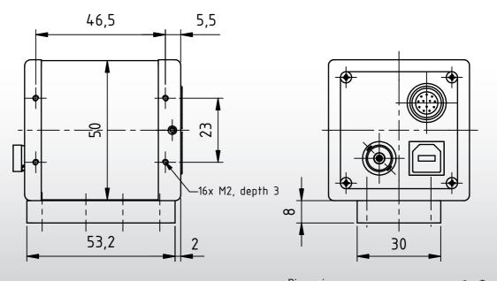
Dimensions: mm Tolerances: DIN ISO 2768m
