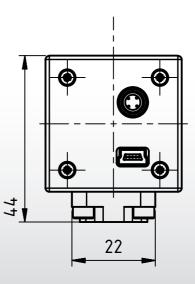
Dimensions: mm Tolerances: DIN ISO 2768m
