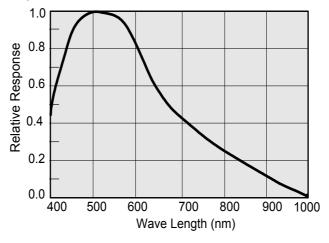
Fig. 27. Spectral sensitivity.
