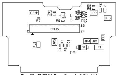
Fig. 28. PK8304 Rear Board of CV-A11
