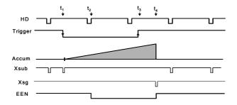
Fig. 16. Pulse Width H asynchronous accumulation.
