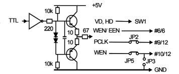
Fig. 7. HD, VD, PCLK, WEN and EEN output.
