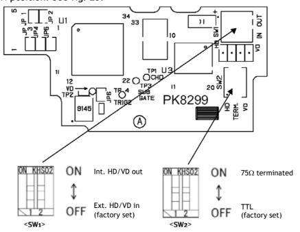
Fig. 26. HD/VD witch positions on PK8299.
