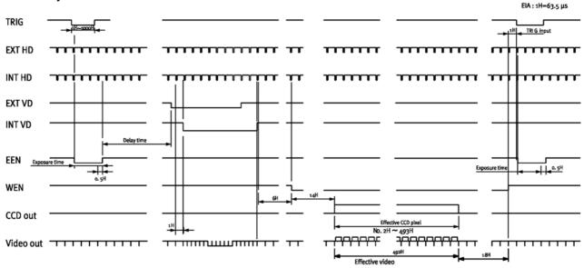
Fig. 19. Frame delay read out
