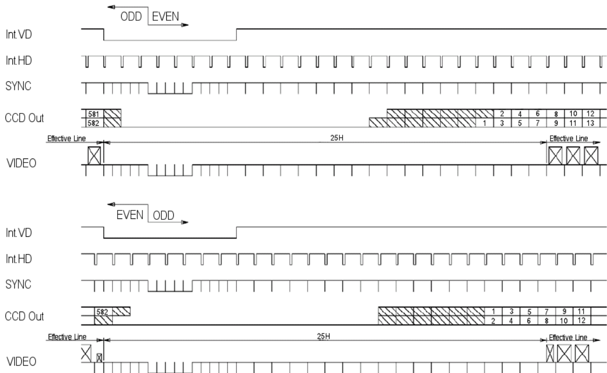
Figure 8. Vertical timing details for interlaced. PAL
