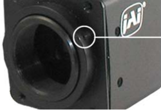
Figure 3. Back Focus Set-Screw Locations
