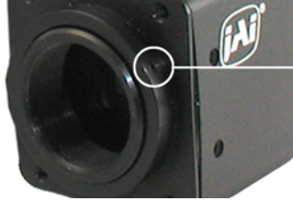
Figure 3. Back Focus Set-Screw Locations
