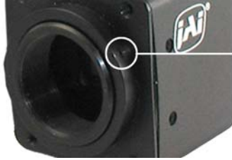
Figure 3. Back Focus Set-Screw Locations
