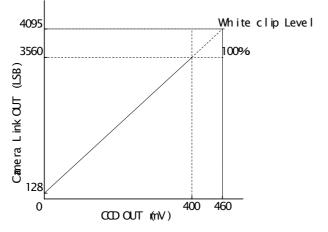
Fig.6. Digital Output Bit Allocation (In case of 12 bits)
