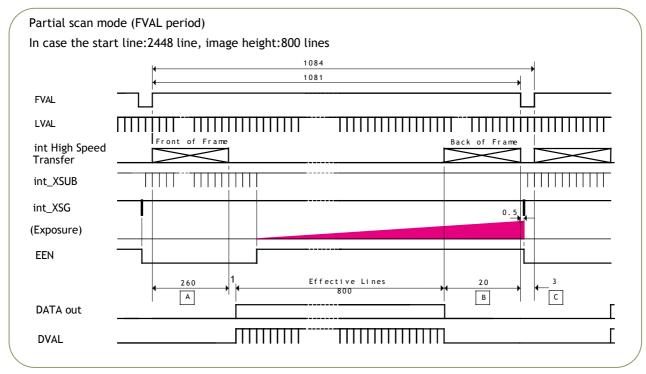
Fig.15. Partial scan Vertical Timing
