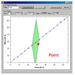
④ Drag the point to a new location within the range or enter new coordinates in the X and Y boxes. Repeat with additional points until the desired response is defined.
