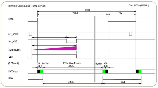
Fig.17. Horizontal Timing for Vertical Binning
