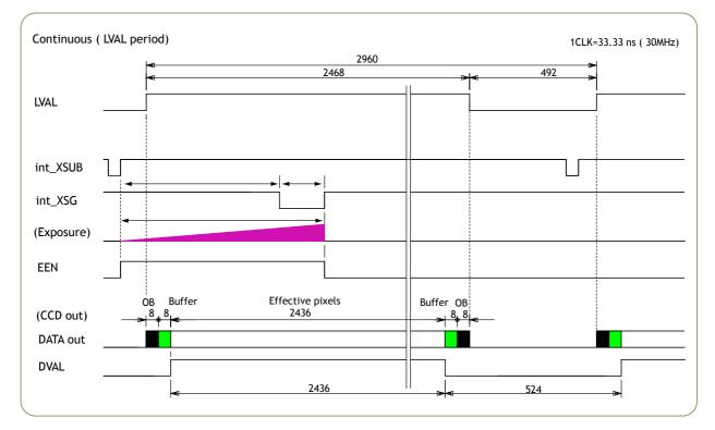
Fig. 13. Horizontal Timing
