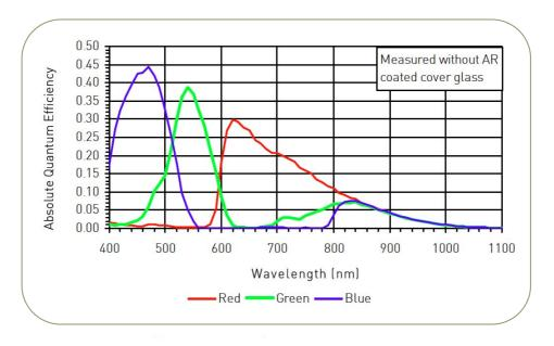
Fig.26. Spectral response for AB-1600CL
