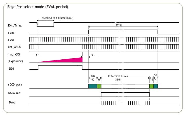
Fig. 19. Pre-select trigger mode.
