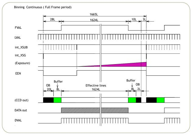
Fig.18. Vertical Timing for vertical binning
