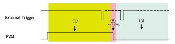
(1) In this period camera executes trigger at next LVAL (prevents feed-through noise)
