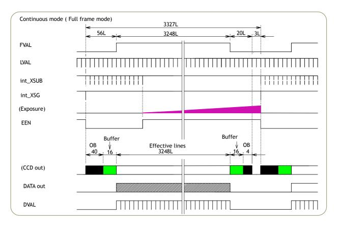
Fig. 14. Vertical Timing for full scan
