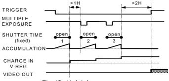
Fig. 13. Multiple exposure
