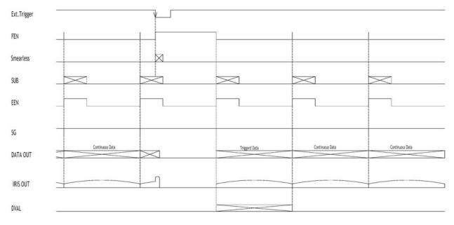
Fig. 21. Edge Pre-select with Restart Continous Trigger.
