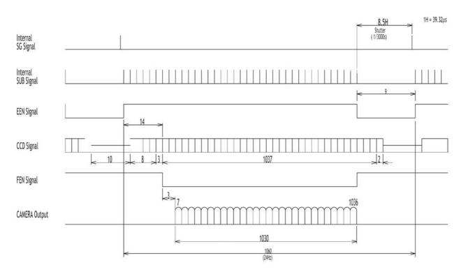
Fig. 17. Vertical timing details, full frame.
