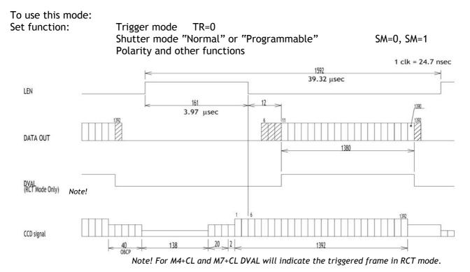
Fig. 16. Horizontal timing details.
