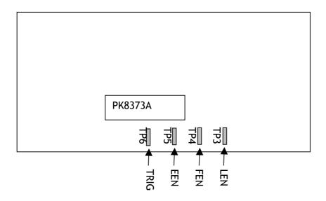
Fig. 32. Camera Link test points
