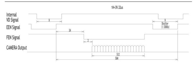
Fig. 18. Vertical timing details with 1/2 partial scanning.
