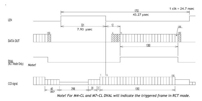
Fig. 16A. Horizontal timing details with V binning.
