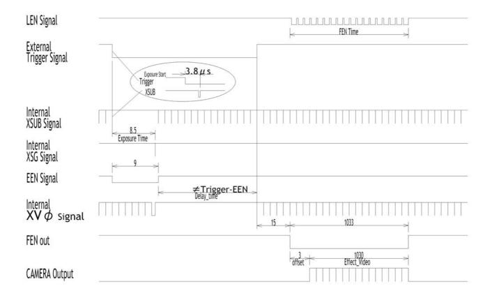
Fig. 23 Frame Delay
