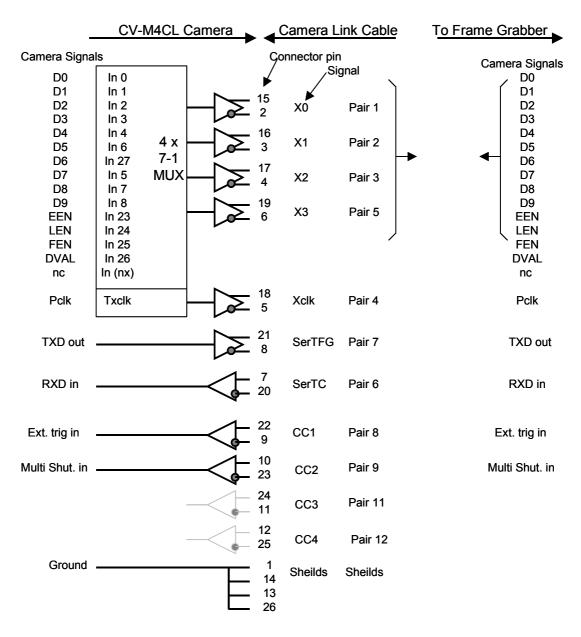
Fig. 8. Principle diagram for Camera Link interface
