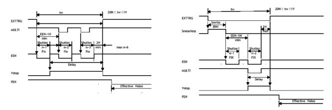
Fig. 24. Multiple exposure, normal and smearless
