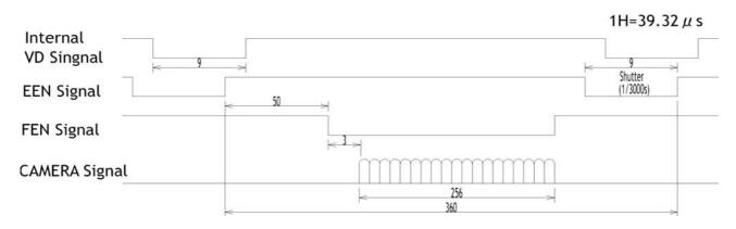
Fig. 18A. Vertical timing details with 1/4 partial scanning.
