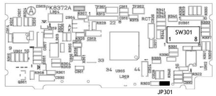
Fig. 27. Internal switch and jumper setting
