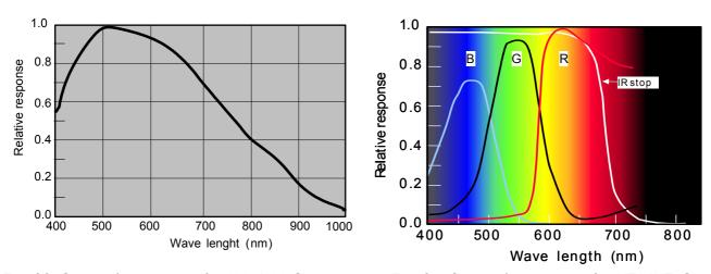
Fig. 30. Spectral sensitivity for M4+/M4+CL
