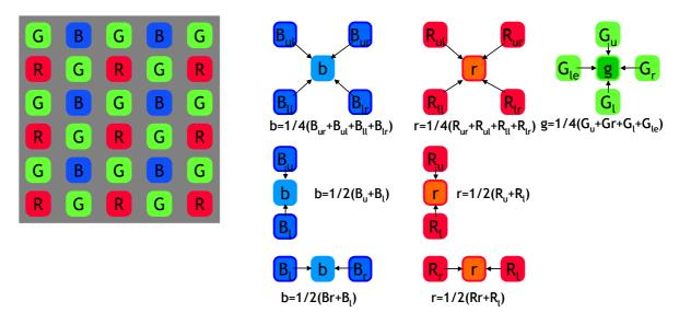
Fig. 14. Color coding from a Primary RGB CCD (Bayer filter)
