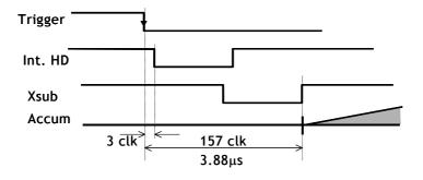
Fig. 19. Accumulation latency time for H a-synchronous trigger.
