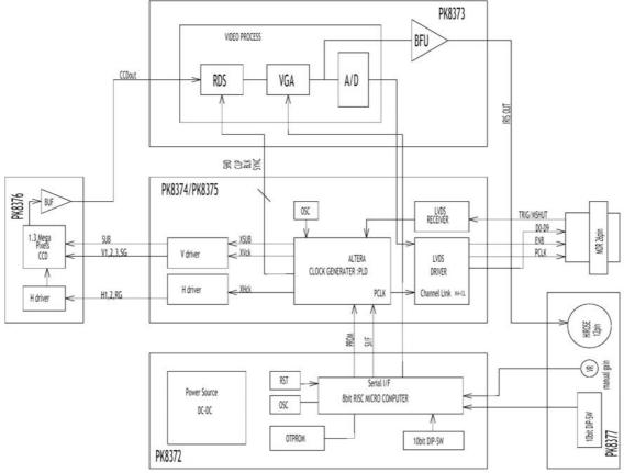
Fig. 9. Block diagram for the camera
