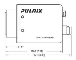
\*A = 18.0 ± 1.0 mm absolute distance measured to front of lens mount (Effective flange back distance = 17.53 ± 0.5 mm)
