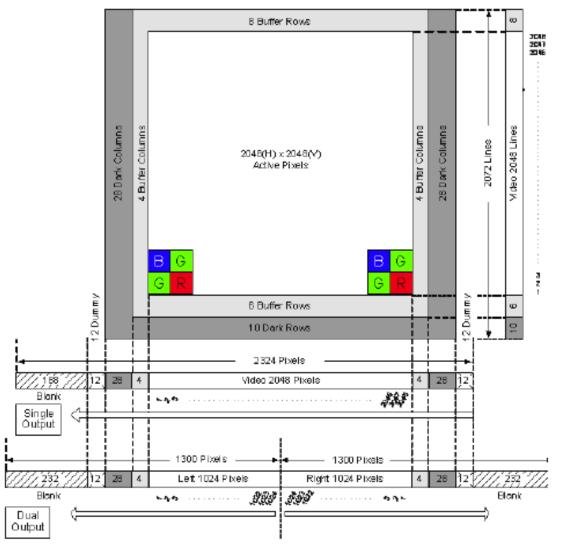
The CCD sensor layout is shown as it is used in the timing video readout with respect to pixels and lines. For the RMC-4200CL the effective full frame Bayer sequence starts with GRG. For partial scan the sequence starts with GRG for the odd lines, and BGB for the even lines.
