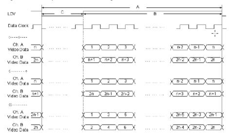
Figure 12. Field Video Timing--Continuous Mode
