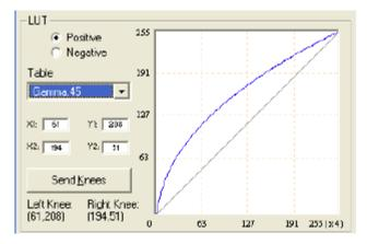
The knee setting allows two adjustments in the light gathering configuration of the LUT to permit the camera to correct images as they are captured. It is possible to set knees on any of the drop down settings by clicking on the existing curve and moving it to the desired configuration. If a drop-down menu setting is selected without adjusting the knees, the camera sets the default.
