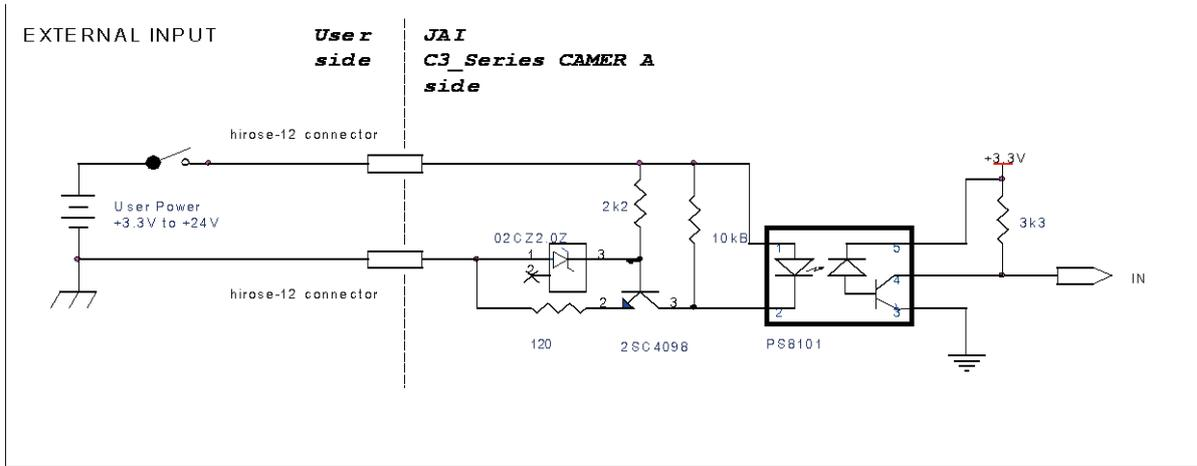
Fig.10 External Input Circuit, OPT IN 1 and 2
