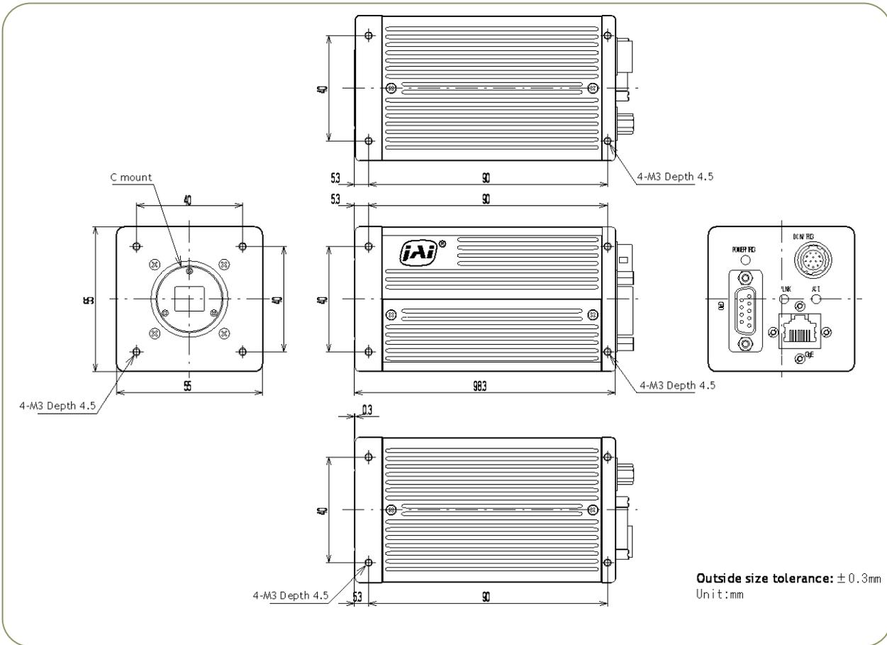
**Note:** Rear protrusion on C-mount lens must be less than 4.0mm
