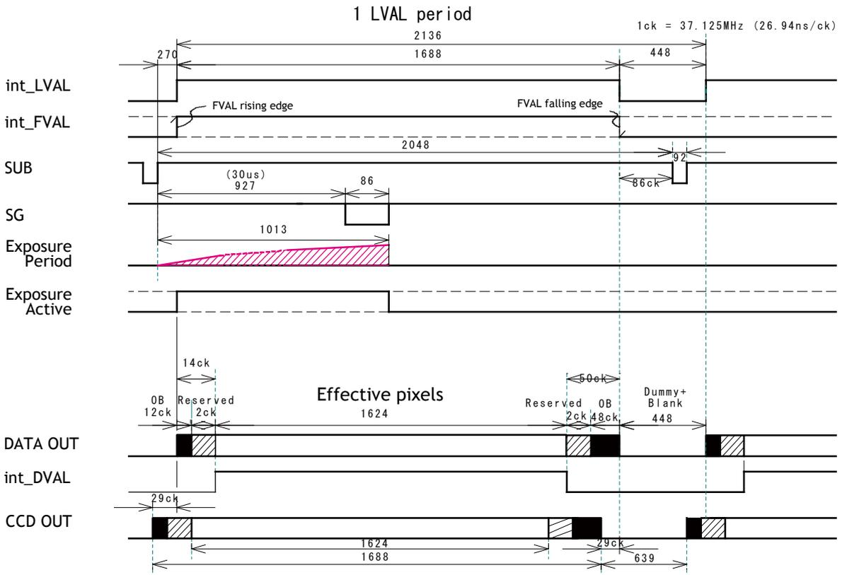
Fig.26 Horizontal timing in Binning Vertical ON
