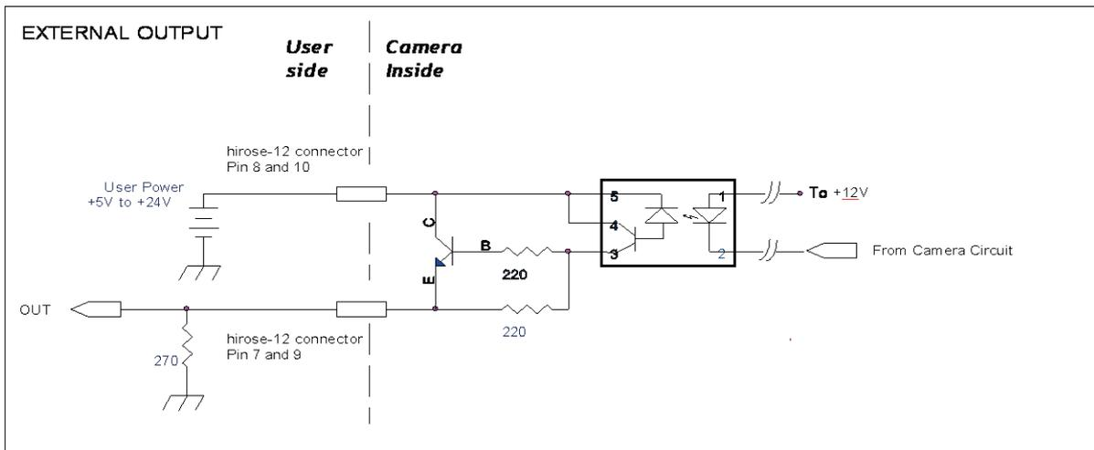
Fig.11 External Output Circuit, OPT OUT 1 and 2
