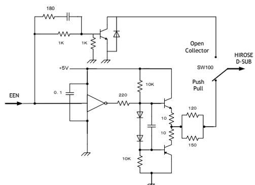
Fig.15 ExposureActive output
