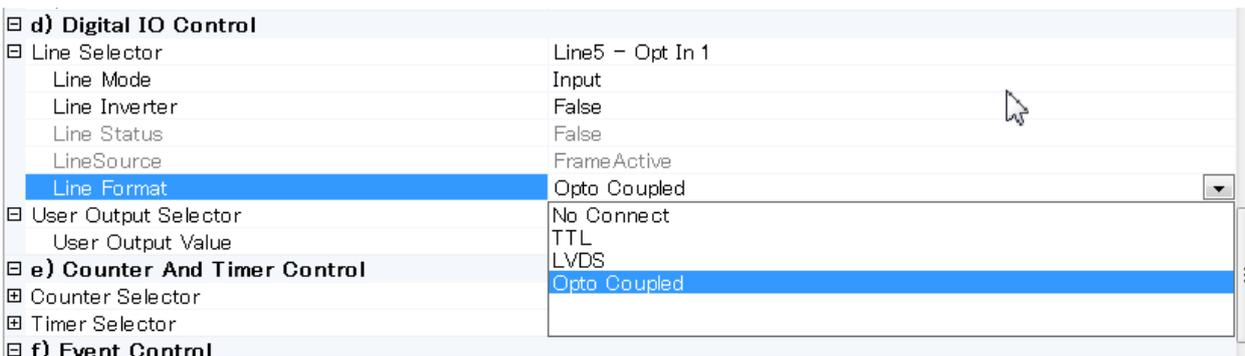
The following figure is an example of setting output so that the signal output from Line1 - TTL Out 1 is selected from signals in the Line Source. In this case, Exposure Active is selected to output through TTL Out 1. TTL is automatically selected as Line Format.
