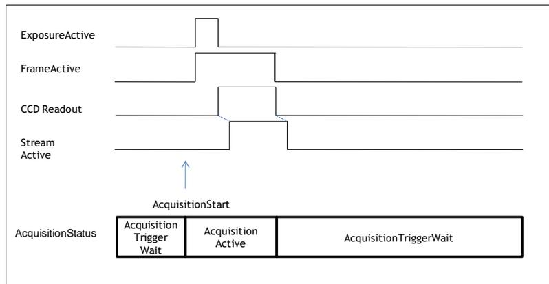
**Fig.28 Single frame timing**
