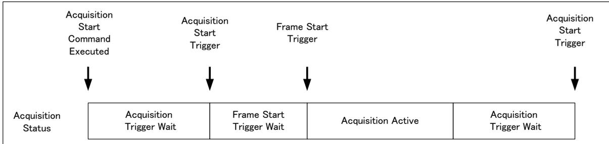
If the acquisition start is set at OFF (The acquisition is controlled internally)
