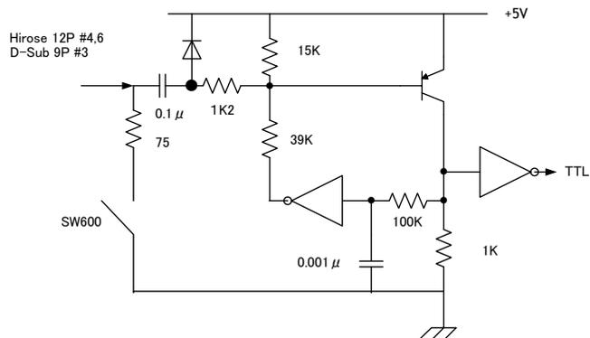
Fig.14 Trigger input.
