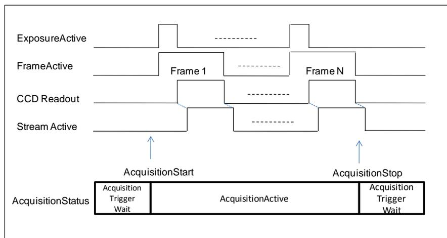
Fig.30 Continuous timing
