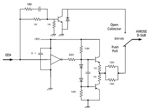
Fig.15 ExposureActive output
