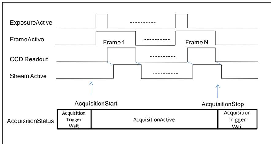
Fig.30 Continuous timing
