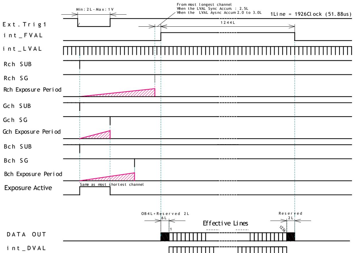
Fig. 37 Trigger control by Timed (Full pixels readout)
