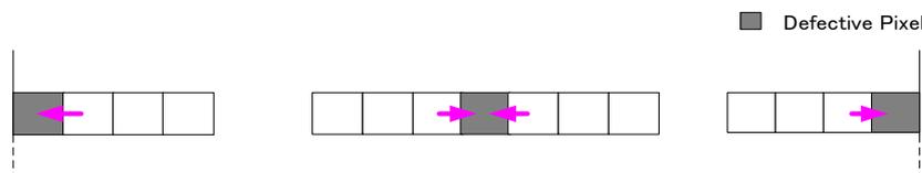
Fig.50 Conceptual drawing for blemish compensation
