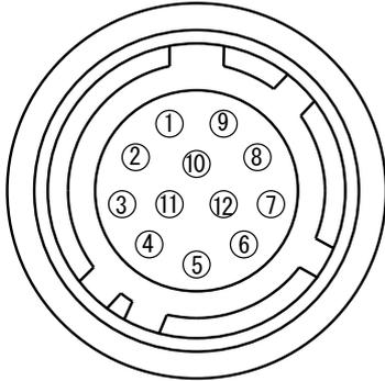
Fig. 3. 12-pin connector.
