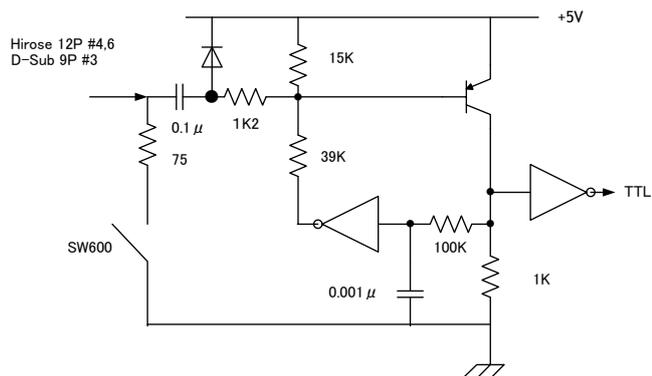
Fig.14 Trigger input.
