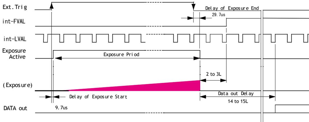
Note: In BinningVertical, the delay of exposure end is 57.54μsec. (1L=2136clock)
