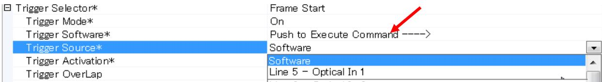
Select “Software” in the Trigger Source and execute Trigger Software command. Software trigger is generated inside the camera and the settings are not changed. Therefore, it is useful if the customer tests the trigger function.
