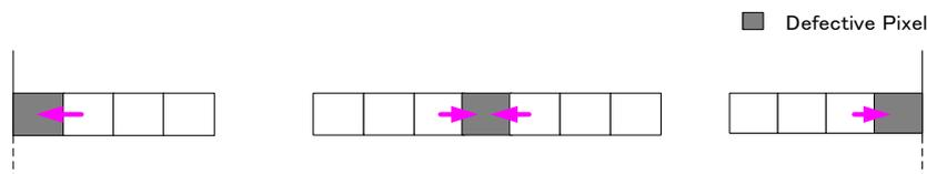
Fig.50 Conceptual drawing for blemish compensation
