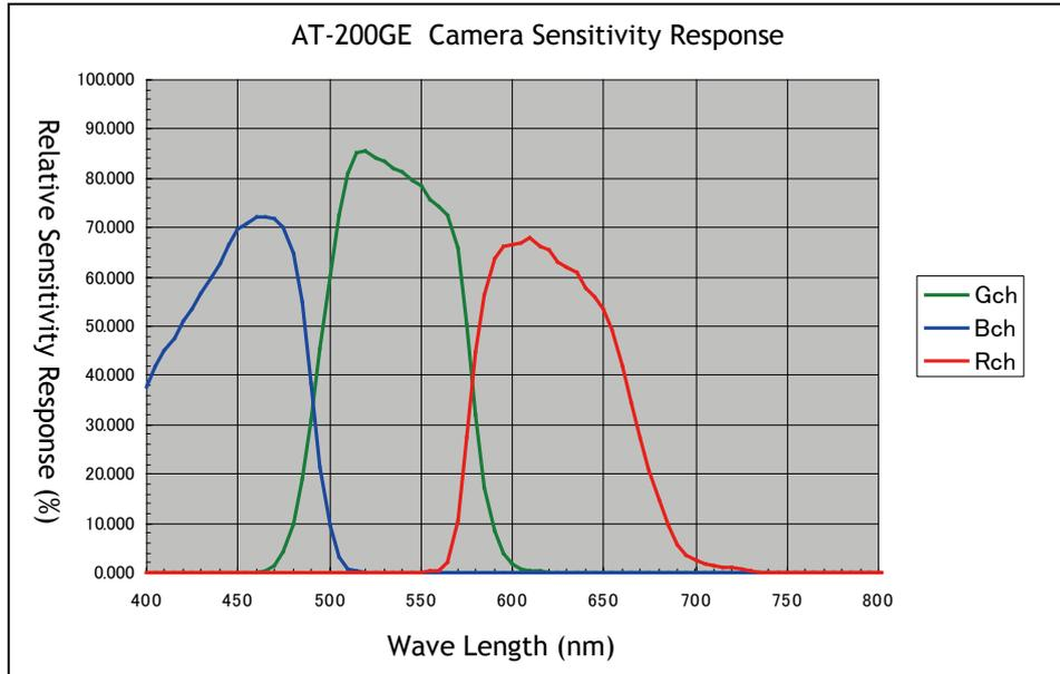
Fig.54 AT-200GE Camera Sensitivity response
