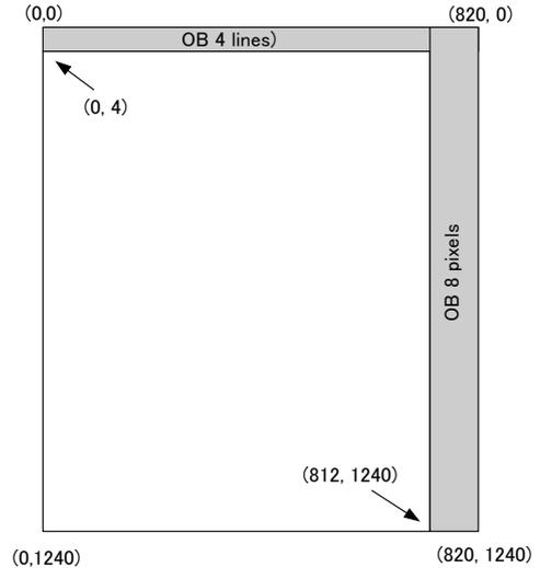
Fig.20 Horizontal binning
