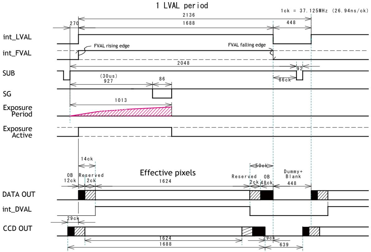
Fig.26 Horizontal timing in Binning Vertical ON
