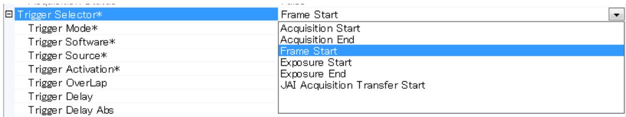
Trigger Selector includes Acquisition Start and Acquisition End commands which determine the start point and end point of acquisition, and Trigger commands which set the trigger timing.
