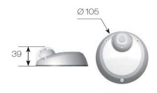
Diagram of mounting holes (unit in mm):
