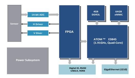
The main components of Woodpecker1 camera includes: Sensor, FPGA and CPU.
